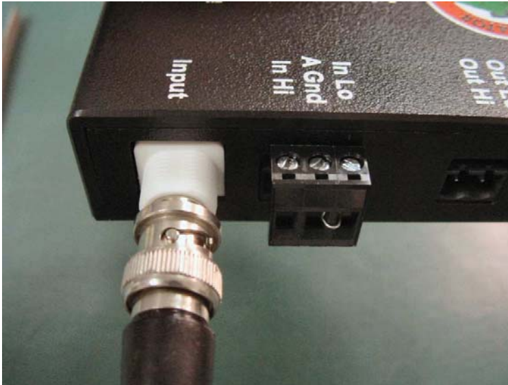
Figure 3-3 Single-ended connection with BNC and wire shunt
