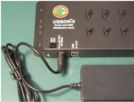
Figure 14-1 Powering the USBDR-8 from the supplied AC adapter
