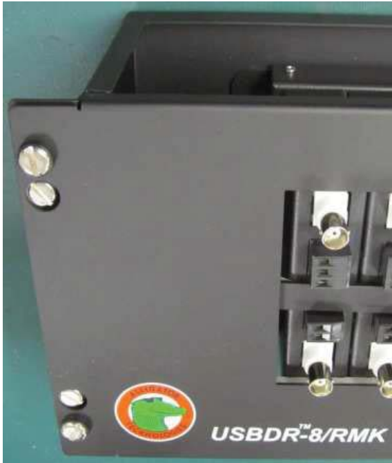
Figure 14-8 first secure the base assembly to the rack with the inset rack bolts and then secure the face plate to the rack mount assembly with the supplied rack bolts and plastic washers.
