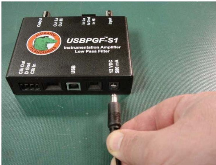
Figure 2-1 Connecting Power to the USBPxx-S1
