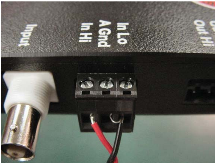
Figure 3-4 Single-ended connection with ground shunt
