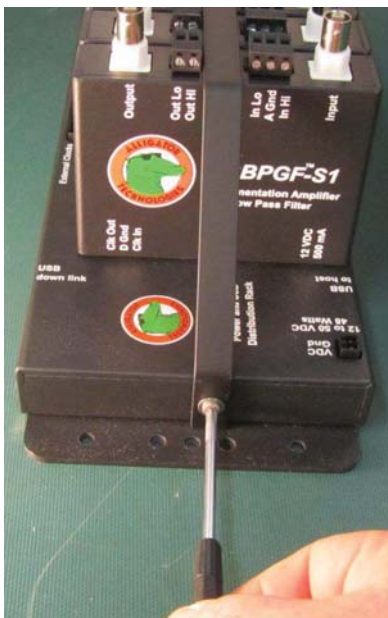
Figure 14-4 Use the supplied washer and screws to securely fasten the hold down bracket to the USBDR-8
