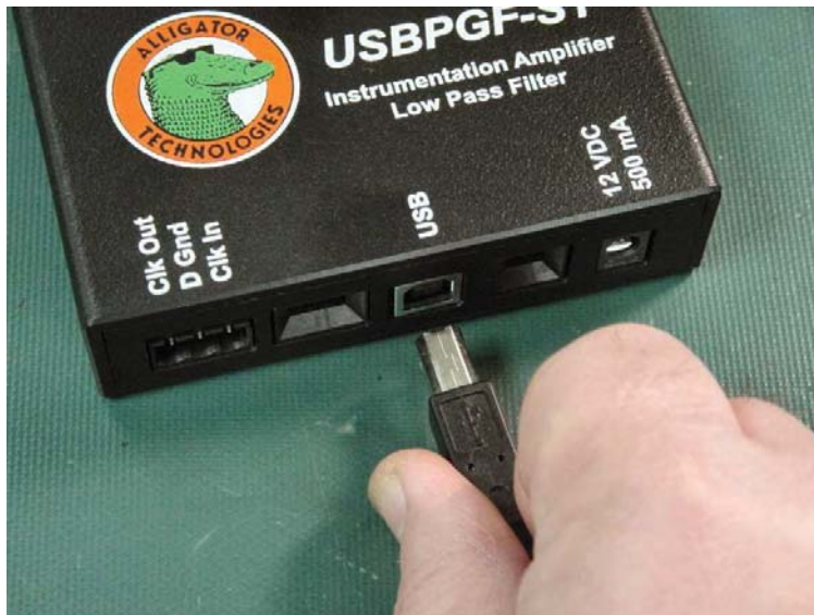
Figure 2 2 Connecting USB to the USBPxx-S1
